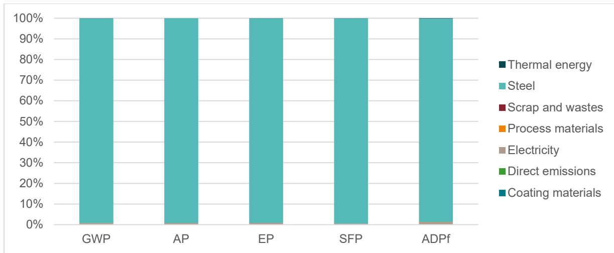
Figure 2: Relative contribution by manufacturing component for 1 metric ton of un-fabricated hollow structural sections
